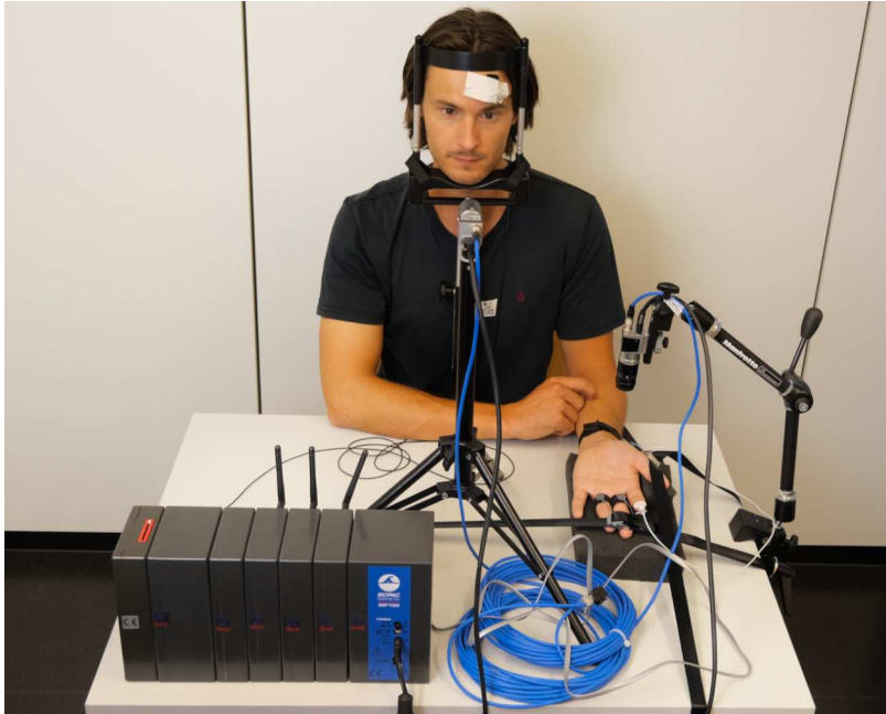
Fig. 2. The overall setup of the study. The face and the palm of each participant are recorded using a Basler acA1300-200uc camera. The participant's EDA signal is recorded on the fingers (ring and middle finger) of the non-dominant hand using two electrodes, and the two PPG signals are recorded on the forehead and at the index finger of the non-dominant hand. The participant uses the dominant hand to pinch the back of the non-dominant arm or the legs as a stressor to cause a spike in EDA. To minimize motion artifacts, the participant's head is placed on a chin rest, and the thumb, middle finger, and ring are placed under a belt such that they do not interfere with the physiological measurements.
